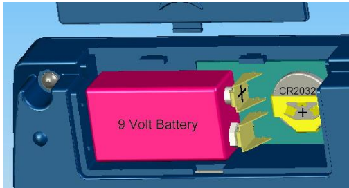
Figure 7: Battery Installation and Replacement
