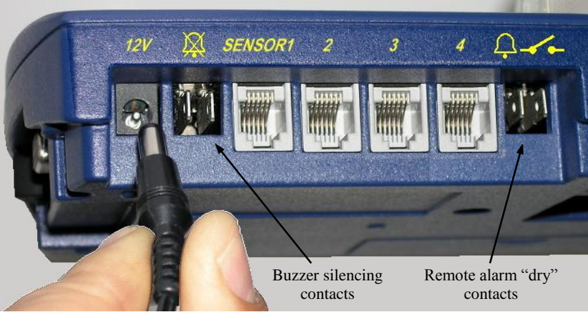
Figure 8: Rear Panel Close-Up
